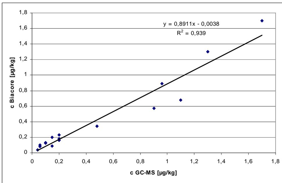
**Fig. 2:** Comparison of screening (Biacore) and confirmatory (GC-MS) concentration results for positive samples (n = 17)
