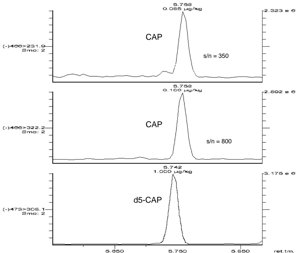
**Fig. 1:** GC-MS/MS (NCI) chromatograms (selected transitions) and signal-to-noise (s/n) ratios of honey sample no. 8, containing approximately 0.1 µg/kg chloramphenicol (CAP) and 1 µg/kg of the internal standard d5-CAP
