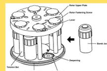
1 g of honey in 3 ml HNO<sub>3</sub> (65% min) in pressure vessel MF 100
