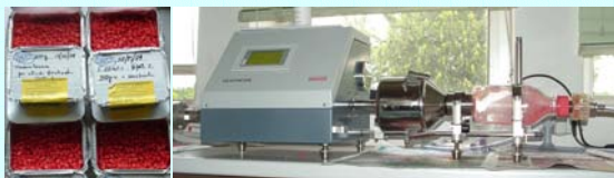
Figure 1 – Dressed seeds (left) and Heubach dustmeter (right) used for the measurement of seed dust.
