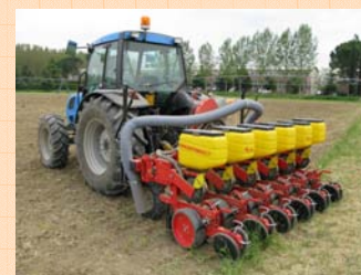
Figure 2 – Seed drill equipped with "dual pipe deflector".
