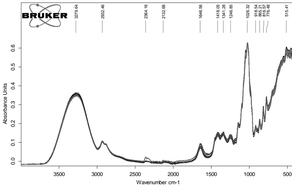
Figure 2 - FTIR- ATR spectrum of the average spectra from honeys acquired from 4000 to 450 cm<sup>-1</sup>.
